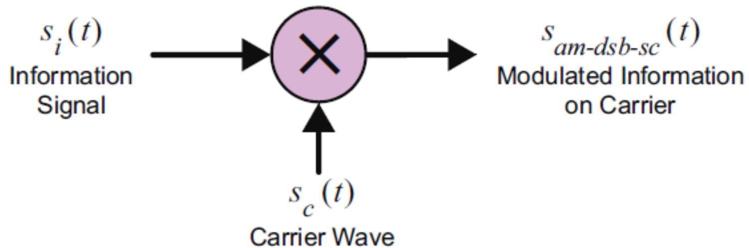
$$s_i(t) = A_i \cos(2\pi f_i t) = A_i \cos(\omega_i t) \quad s_{am-dsb-sc}(t) = A_i \cos(\omega_i t) A_c \cos(\omega_c t)$$
