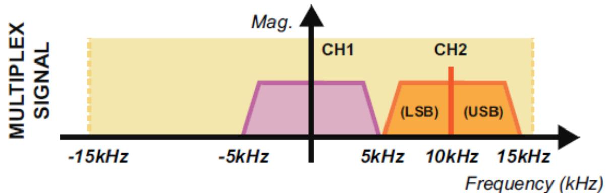
If another complex carrier (this time with a frequency of -10kHz) was used, it would be possible to position another channel in the negative part of the double sided spectrum.
