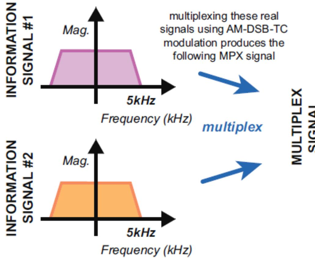
When the 10kHz carrier used to AM-DSB-TC modulate information signal 2 into channel 2 is real, the baseband MPX signal is symmetrical when plotted as a double sided spectrum
