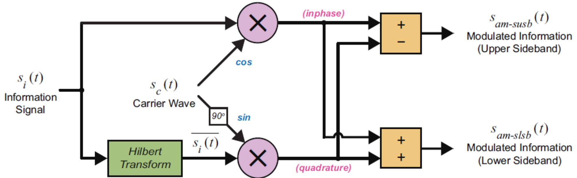
$$s_{am-ssb}(t) = s_i(t) \Re e[s_c(t)] \mp \bar{s}_i(t) \Im m[s_c(t)]$$
