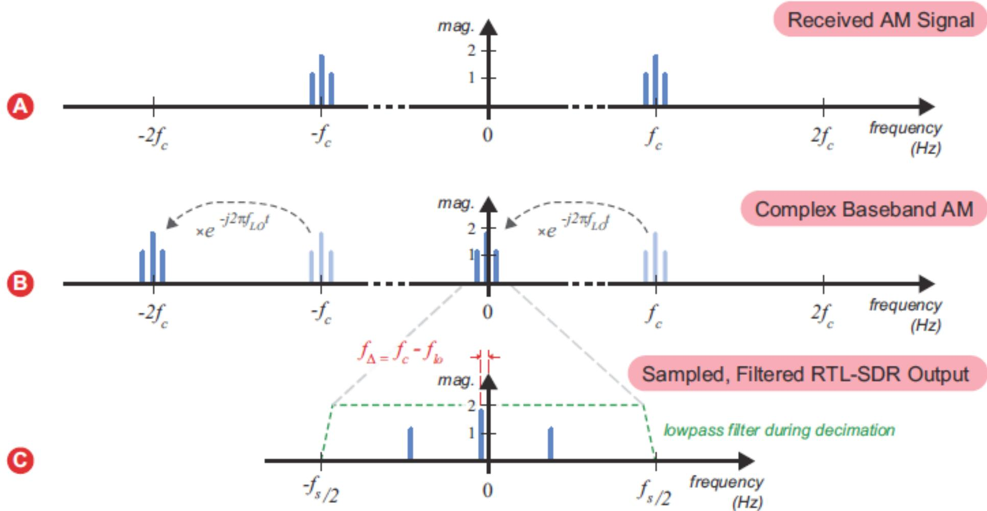
$$s_{amRF}(t) = s_{am-dsb-tc}(t) = A_o A_c \cos(\omega_c t) + \frac{A_i A_c}{2} \cos(\omega_c - \omega_i)t + \frac{A_i A_c}{2} \cos(\omega_c + \omega_i)t$$
