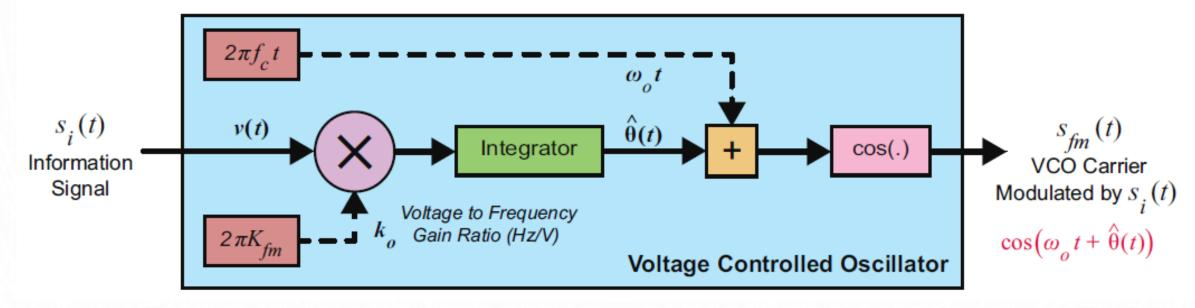
$$\hat{\theta}(t) = k_o \int_{-\infty}^{t} v(t) dt \qquad \hat{\theta}(t) = \theta_{fm}(t) = 2\pi K_{fm} \times \int_{-\infty}^{t} s_i(t) dt \qquad c(t) = A_o \cos\left(2\pi f_o t + \hat{\theta}(t)\right)$$
