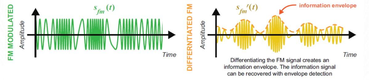
The fluctuations in this envelope are directly proportional to the instantaneous frequency
